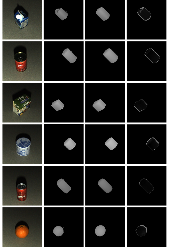
Figure 6: Visual examples of the fitting performance of the proposed CNN regressor with real-world data, captured by the Artec MHT 3D scanner. Results are shown for all 6 scanned objects (in rows). The column show (from left to right): the scanned object in RGB, the rendered range image in an isometric projection, the estimated superquadric, and the absolute difference between the range image and superquadric representation.
