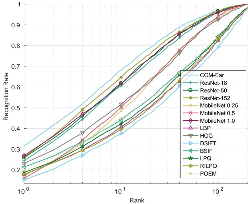
Fig. 3: CMC curves of the comparative evaluation of the COM-Ear Model. The results are presented in logarithmic scale to better visualize the performance differences at the lower ranks, which are more important from an application point of view. The figure is best viewed in color.
