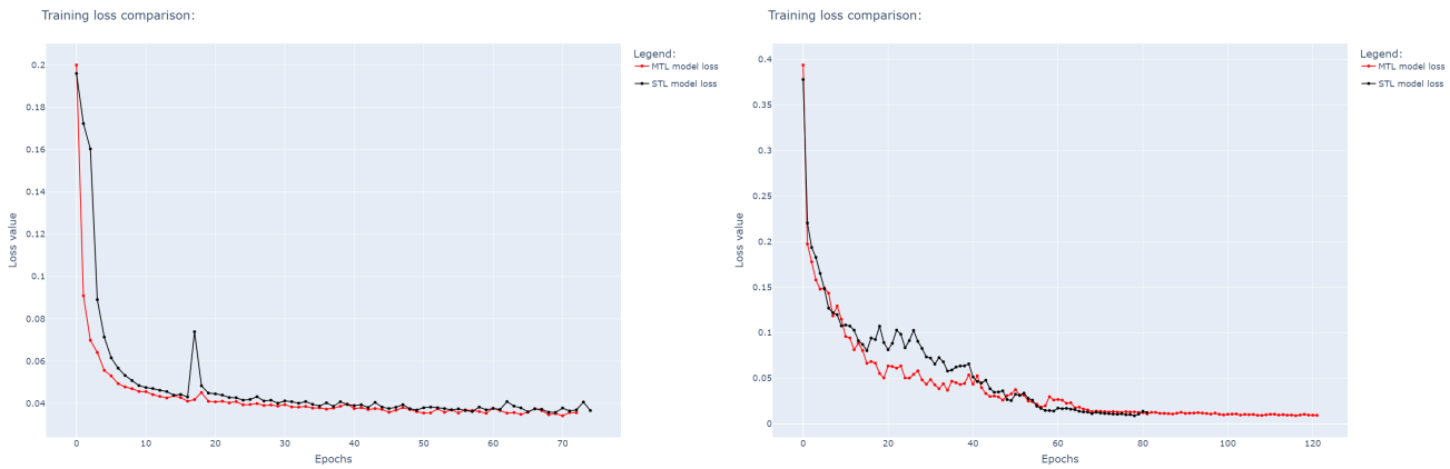
Figure 7: Comparison between the loss function values for single-task (black) and multi-task (red) learning models, first for the MOBIUS dataset, followed by the values for the SBVPI dataset on the right.
