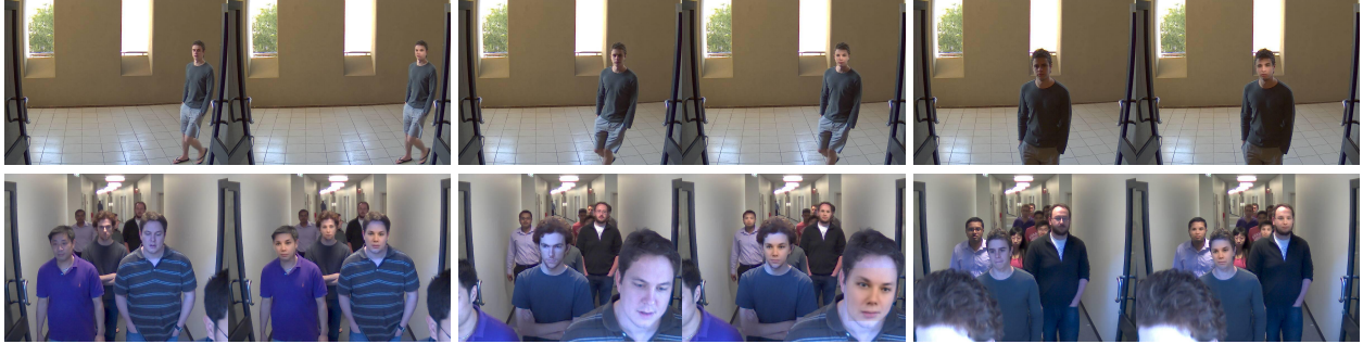
Fig. 6. Qualitative examples of problematic deidentification results. The upper row shows an identity switch in the last frame due to a change in the scenes illumination. The lower row shows difficulties due to the presence of multiple people, some of which occlude faces in the background. Misalignment between the original and surrogate faces is also visible in the second image pair of the lower row, which happens due to extreme viewing angles when people exit the scene.
