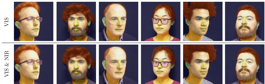
Fig. 16 Segmentation improvements when utilizing bimodal (VIS & NIR) instead of unimodal (VIS) data. Two DeepLab-V3 models are trained on privacy-preserving synthetic data of BiFaceGAN, either on the VIS data or on the entire VIS & NIR data pair. Performance is then evaluated on the validation part of the Tufts Face dataset [22].
