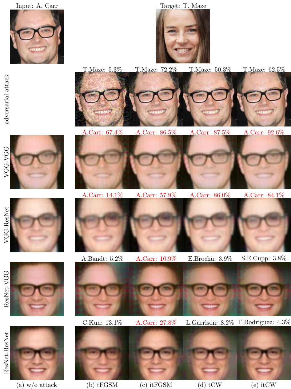
Figure 12: Adversarial attack results without (row 2) and with (rows 3-6) the use of DFD reconstructions. Predicted identity above each image. Adversarial attack designed to fool the system into classifying A. Carr as T. Maze. DFD reconstructions show resistance to adversarial attacks, especially when reconstructing from the VGG embeddings. ResNet-based reconstructions (bottom two rows) also exhibit some characteristics of the target gender. Each column is a different attack method: (b) targeted FGSM, (c) iterative targeted FGSM, (d) targeted CW, (e) iterative targeted CW.
